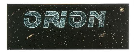
At its most basic level, a fiber optic display can appear almost as a series of reflector buttons on a highway sign. Photo courtesy of G&B Optics, Las Vegas, NV.
